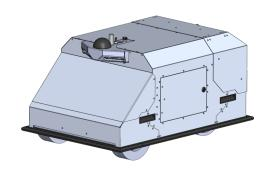
Angsa revolutionizes the removal of trash on grass and gravel: Individual objects are detected by an artificial intelligence and removed by the autonomous robot.
